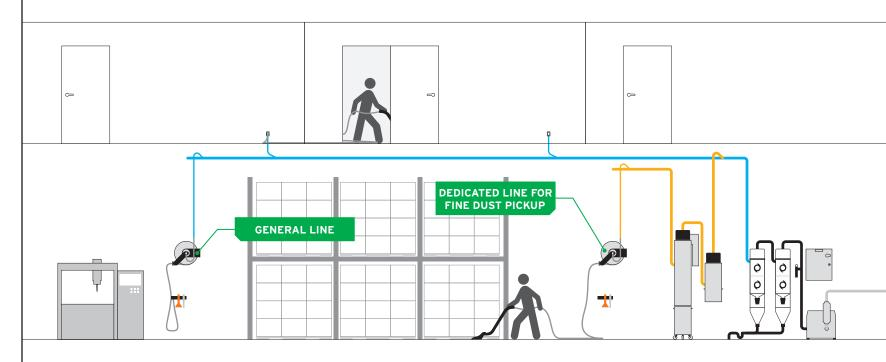
Custom-made Industrial Automatik with **fine dust separator** and **VacReel**®
